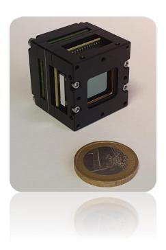
**IrLugX320P** is a simple and immediate solution for integrators of handheld infrared devices (such as monocular, binocular, head-up displays). It can also be the reference design to be customized and become the handheld core part of the finished end-product of system integrator.
